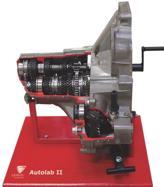
This trainer provides the instructor with a complete manual gearbox for group or whole-class demonstration, mounted on a steel plate for use on a workshop bench or classroom desk. The gearbox is operated by hand and is sectioned so that all moving components can be seen and the way they interact can be observed.
