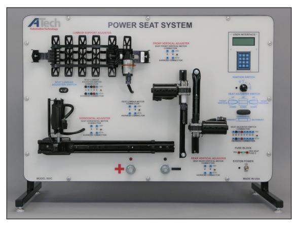
The ATech Power Seat Trainer (model 860C) is part of an electrical system program which presents the live operation and study of power seat systems. This trainer allows for instructor demonstration, student hands-on reinforcement and troubleshooting practice. Powered by a 12VDC automotive battery or 12VDC/30A power supply (not included). The Power Seat System is based on a CAN platform vehicle.
