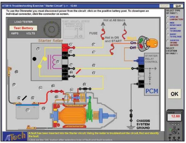
The Starter System Troubleshooting Trainer is a software program based on a Starting System and deals with the basic concepts of troubleshooting those automotive components. This program can operate in Random Mode, where the faults are selected randomly for each circuit chosen, or the instructor can select faults from various circuits to be activated as each student runs the program.
